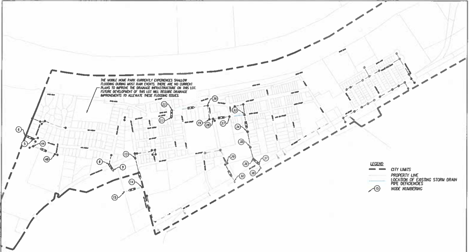
FIGURE 3 EXISTING STORM DRAIN PIPE DEFICIENCIES
