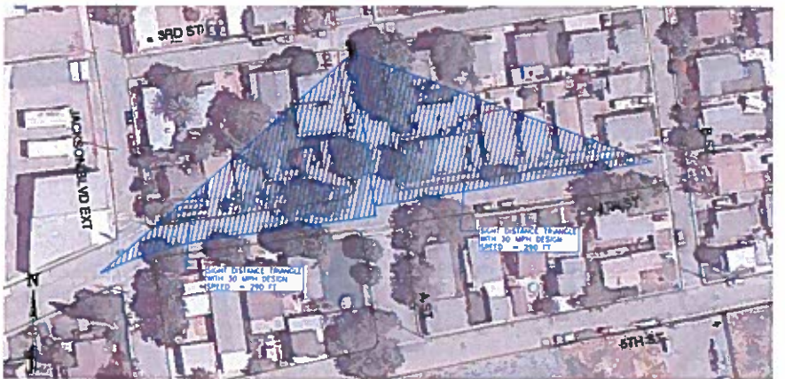
SOUTHBOUND APPROACH - CASE C1 (CROSSING MANEUVER FROM THE MINOR ROAD WITH YIELD CONTROL)
