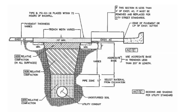
NOTE: CONTINUOUS TRENCHES MORE THAN 500 FEET IN LENGTH AND WHERE THE TRENCH LIES WITHIN A TRAVELED LANE, THE ENTIRE WIDTH (12 FEET MINIMUM) OF THE LANE, SHALL BE OVERLAID WITH ASPHALT CONCRETE. PER THE CITY INSPECTOR.
